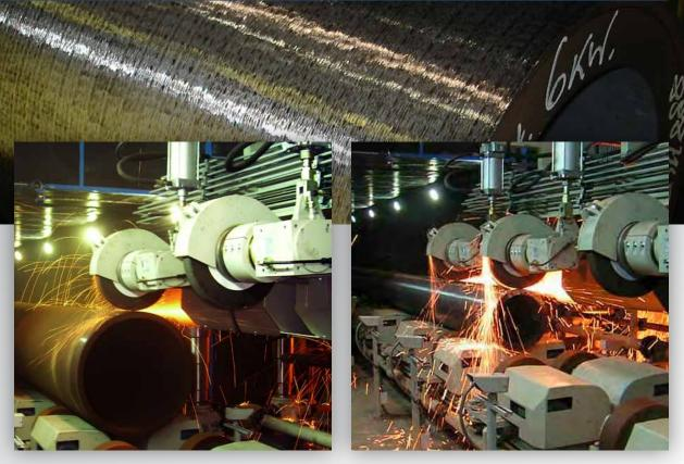
Our tube grinding machines are ideal for pre-treating rolled, forged and drawn thick-walled tubes. The surface is rough ground for subsequent machining.
