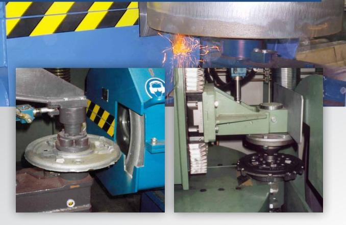
The simple, rugged and foundry designed build of our cylindrical grinding machines, ensures a high system availability. Cylindrical grinding machines are perfectly suited for the fettling and removal of joint surfaces at cylindrical castings with diameters of either 150-600mm or 200-400mm.
