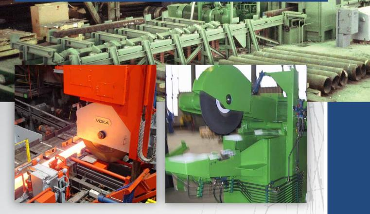
Our high efficient machines are used worldwide in rolling mills and forging plants for the cutting of cold or hot, high alloyed and super alloyed materials. VOKA machines are constructed for the use of wheel dimensions up to the diameter Ø of 1850mm.
